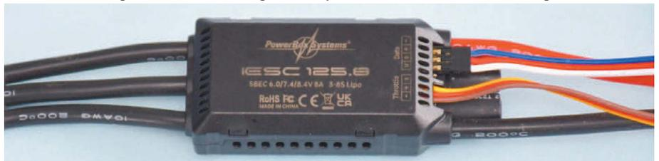
Underside of the iESC, where the connection for the (blue, red and white) telemetry lead and main throttle channel lead can be seen
