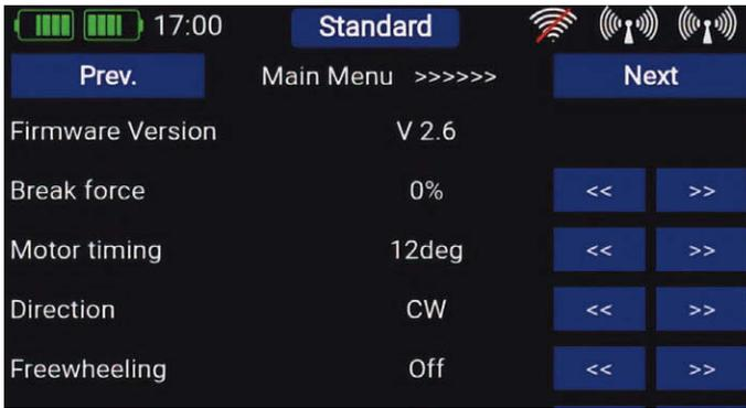
First of the three parameter setting screens on the Atom transmitter
