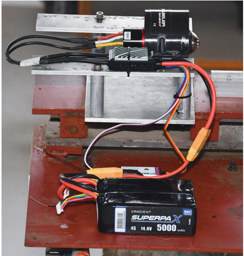
iESC alongside the Schuebeler EDF unit on the test rig, with PBR-9D receiver and battery packs
